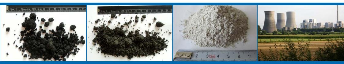
From left to right (Source: MVW): Picture 1 Wet ash from a German lignite power plant, Picture 2 Wet ash from a German hard coal power plant, Picture 3 Fly ash from a hard coal power plant, Picture 4 Hard coal power plant: Cooling towers on the left, generator, boiler house and other facilities on the right hand side
