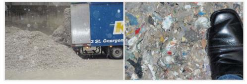
**Picture 1** Unloading "fluff" from a Walking-Floor® truck into the storage hall of a cement plant for kiln burner feeding (left); close-up of the fluff (right) (source: MVW).
