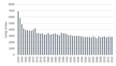
Figure 2 Trend in specific thermal energy consumption, expressed as kJ/kg clinker; numbers up to 1987 reflect only Western Germany, the following years cover entire Germany; numbers according to (4).
