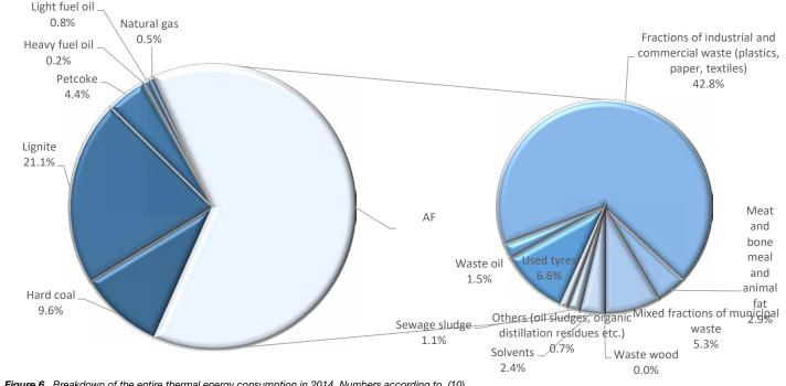
Figure 6 Breakdown of the entire thermal energy consumption in 2014. Numbers according to (10).
