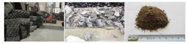
Picture 2 Storage of whole tyres for kiln inlet feeding (left); tyre chips for kiln inlet feeding (centre); animal meal for kiln burner fring (right) (source: MVW).
