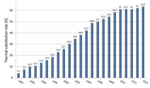
Figure 3 Average utilisation of alternative fuels in the German cement industry in terms of thermal substitution rate; numbers according to (5)
